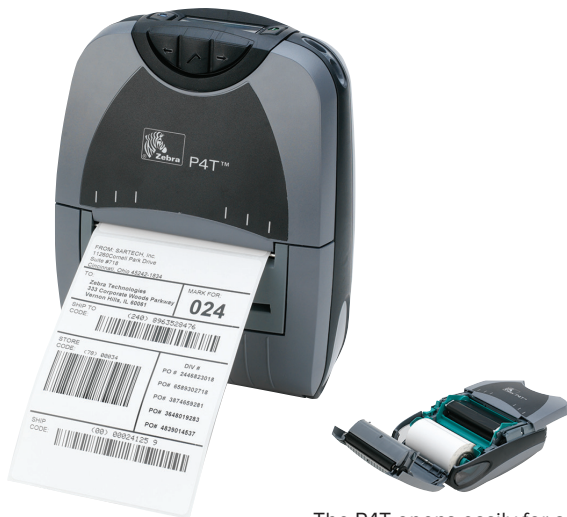
The P4T opens easily for a quick and simple change of media and ribbon cartridge.
